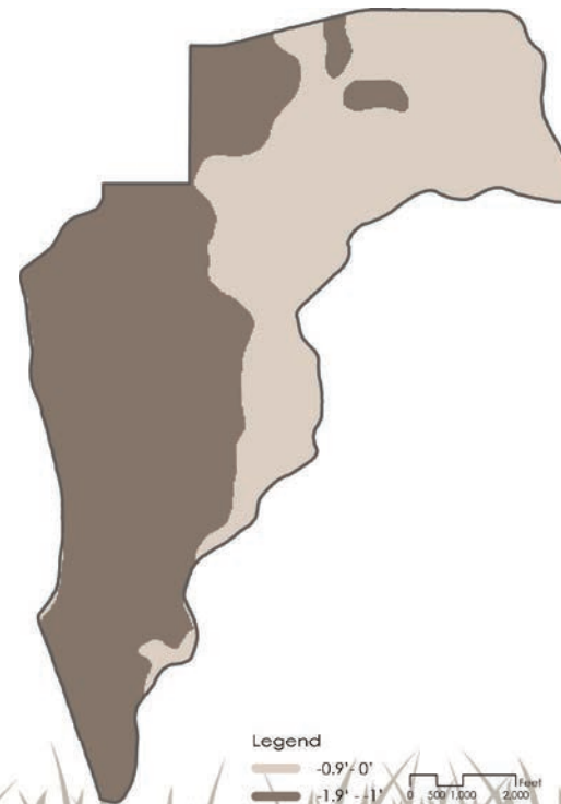
Figure 2.3: Subsidence at MWT
