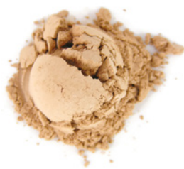
Filtration Sand < 0.7 mm (0.03")
