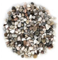
Separating Gravel 0.7 mm (0.03") - 6mm (1/4")
