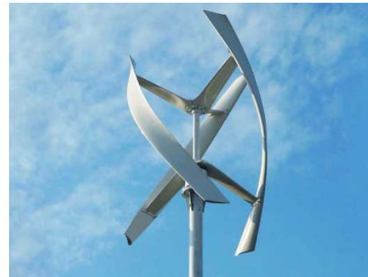
5.3 Vertical-axis wind turbine
