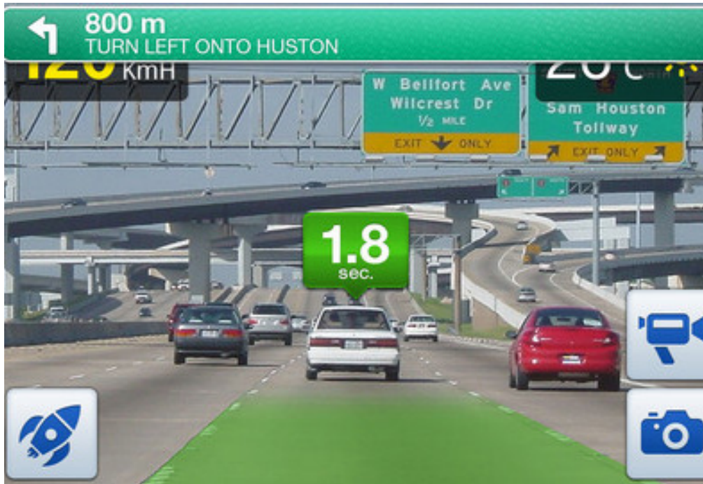
3.12 Screenshot of iOnRoad App, using camera and distance algorithms
