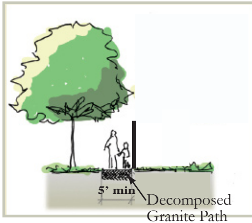
Figure 5.16: Section of DG path
