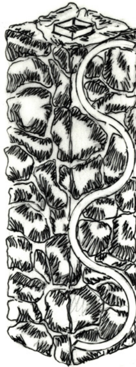
4.1 - Stone Column with Incorporated Metal Wine Barrel Rings
