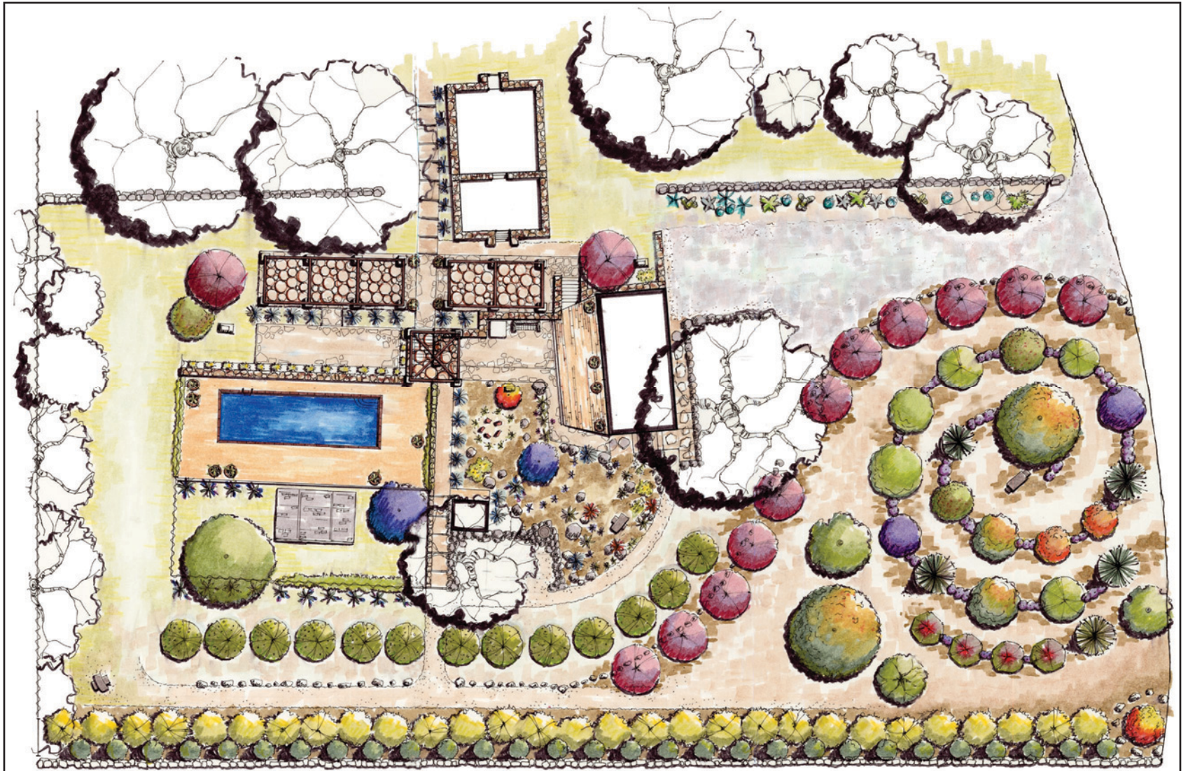
From left: pool and grape arbor, stone patio, vegetable garden, terraced informal planting on slope, pool house, cactus garden, almond curve, spiral fruit orchard. Vegetative barrier: cypress, cryptomeria, almond, olive, flowering shrubs. Original at: 1"=10'-0"
