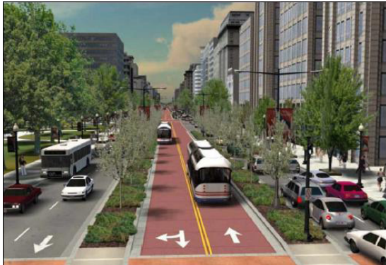
Figure 1.6 Designated Bus-Only Lane can be reduced by providing Transit Signal Priority at intersections (Fig. 1.5). This technology tracks the position of BRT vehicles and extends the green light along the bus' direction provided it's within a certain proximity to the intersection or conversely shortens the length of it's red light when stopped.
