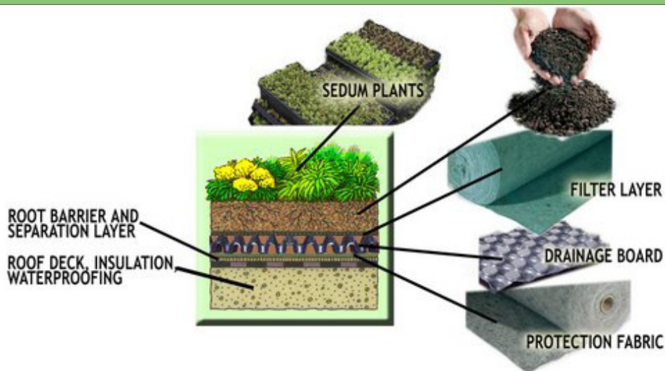
Typical Setup of Extensive Green Roofs. Designed by Jörg Breuning, Green Roof Service LLC
