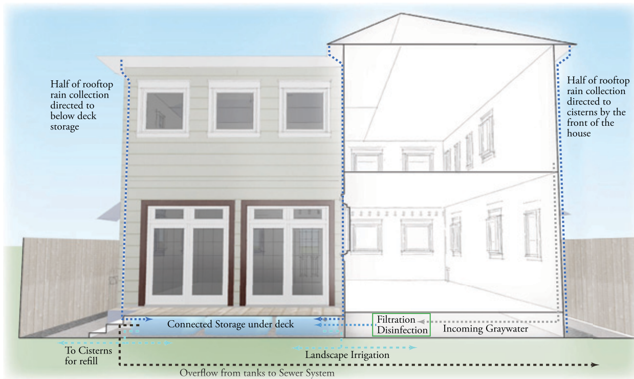
Left: Schematic of graywater and rainwater flows
