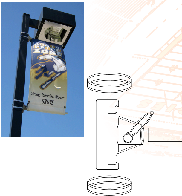
Image 6.6 and 6.7: Some exterior signage exists around Aggie Stadium, however it only designates the Aggie Pride Zone (left). A schematic drawing of the banner “rod-holder” and the fasteners that attach it to the light post.
