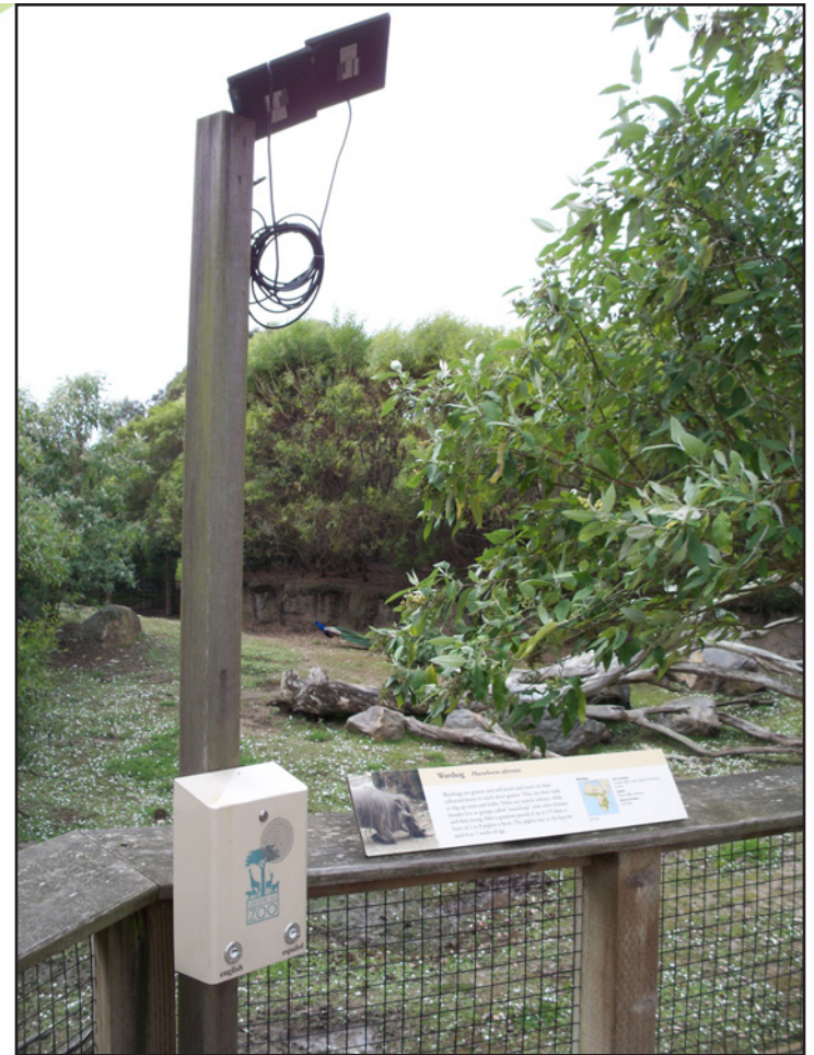
Fig. 4.42: This solar powered information box at the San Francisco Zoo is one simple way to incorporate more sustainable features. It also provides an opportunity for education about implementing such technology at home.
