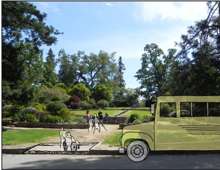
Fig. 4.20: By replacing only two existing steps with an ADA compliant ramp and performing some simple regrading, the entire area becomes accessible to everyone.
