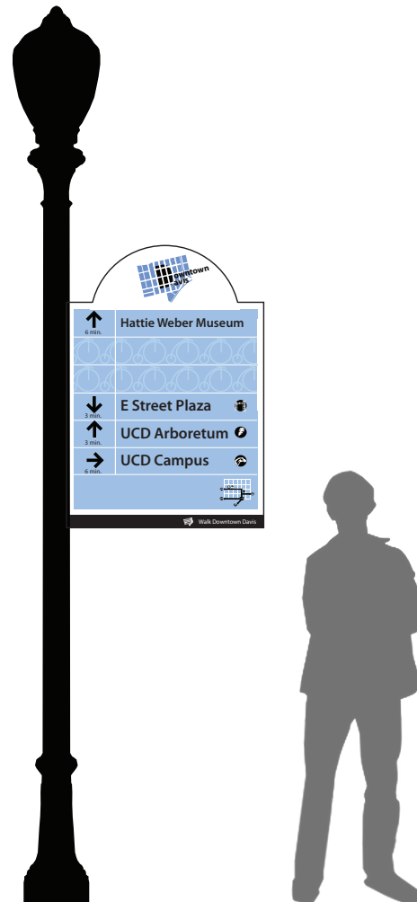
3-22: elevation of directional sign on existing lamppost
