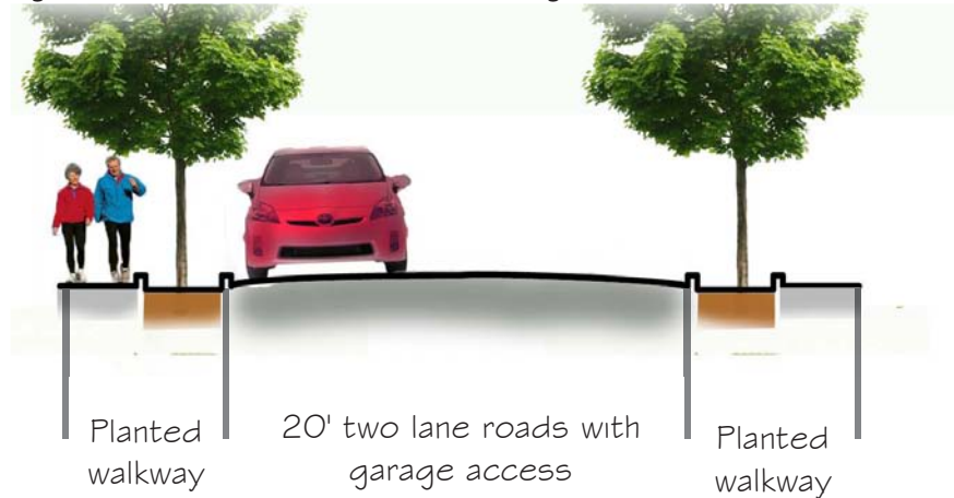
Figure 4.5 Section of streets between housing
