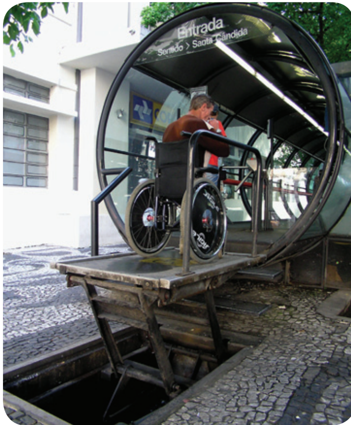
Figure 2.17: Tube accessibility for the disabled.
