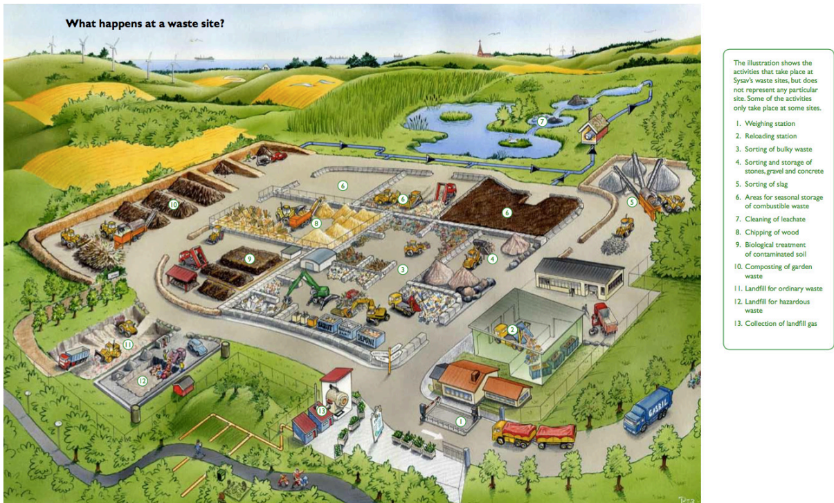
Figure 4.2: SYSAV Waste Recovery Site (SYSAV)
