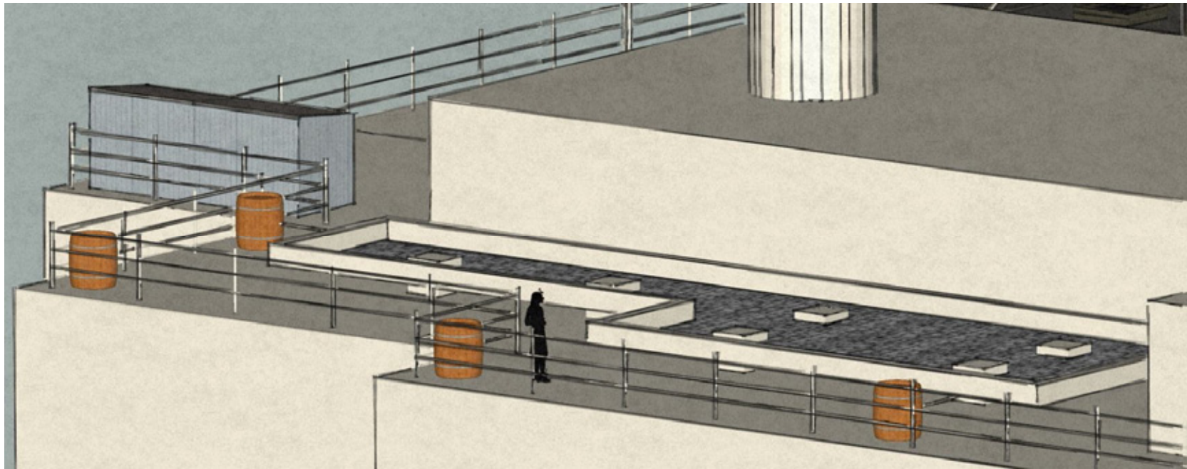
Fig. 5.05: Shallow planter used to collect and filter water for rainwater harvesting.
