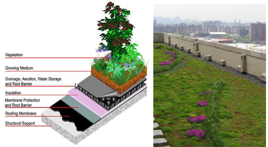
Fig. 2.01: Typical green roof layers (Left). Green roof on the Bronx County Courthouse (Right).
