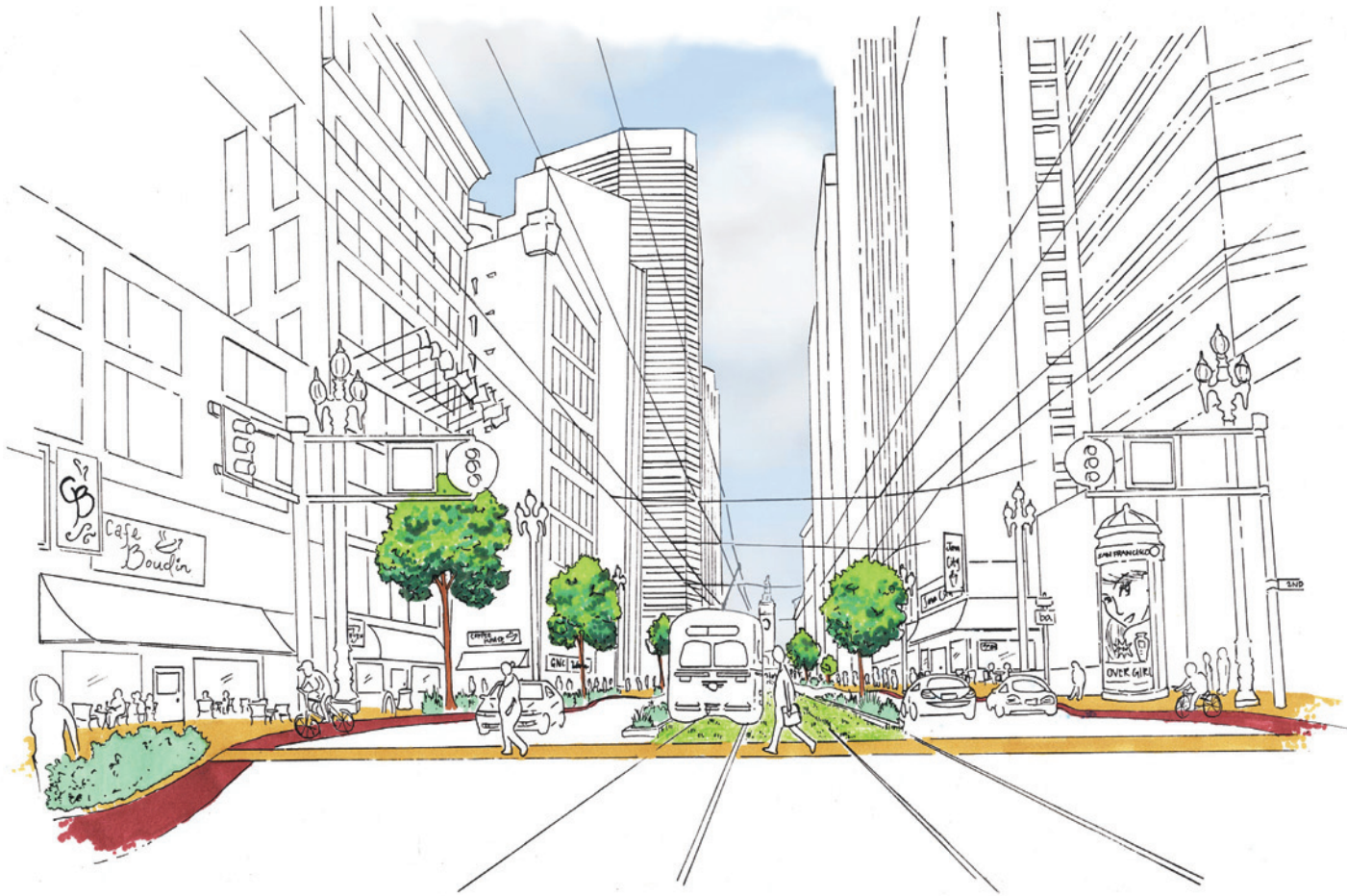
Perspective looking East from 2nd Street: this illustrates new design ideas on Market Street, including colored bike lanes, a green grass median, native species plantings, and outdoor cafes.
