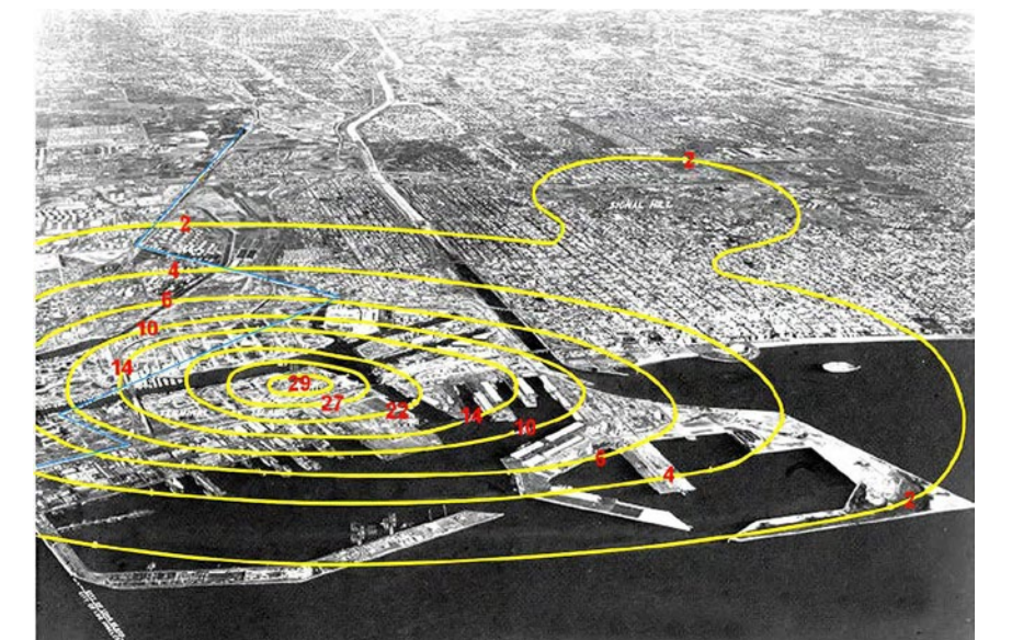
Subsidence affects urban areas too. This is Long Beach, CA subsiding due to oil mining. (Source: Borchers and Carpenter, 2014)
